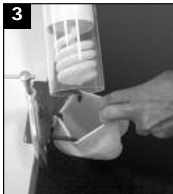
3 Stretch the balloon onto the tool, and insert the balloon bulb unit.
