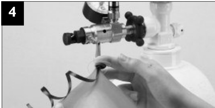
Slide tying disc down approximately one inch on the neck of the balloon.
