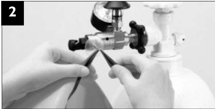
Hold the inflated balloon in your left hand. With your right hand, pinch the neck of the balloon and the ribbon together and stretch both around the end of the tying post.
