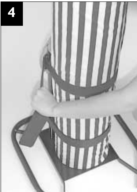
4 Roll the cylinder into the safety stand until it is touching the upright supports. Orient the cylinder valve outlet so it is facing to the left. Place bottom Velcro® safety belt around cylinder and through loop. Tighten belt securely. Repeat with top belt. Cylinder should be very tightly attached to stand.
