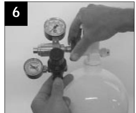
6. Hand tighten the primary regulator to the helium cylinder.
