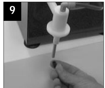
9. Place the inflator near the edge of a clean smooth-surfaced counter. Press down firmly to secure the suction cups on the base of the inflator to counter. Remove blue cap from the Hi-Float® outlet.
