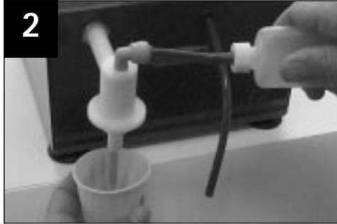
2. Fill the small squeeze bottle with hot water. Insert the blue hose on the end of the squeeze bottle into the helium outlet. Place a cup under the outlet to catch the hot water. Flush the passage with the hot water by squeezing the water bottle. This will dissolve any residual of Hi-Float® and clean the outlet.
