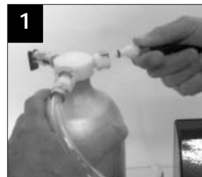
1. Press the silver release tab on the helium supply line to remove the line from the cylinder. Repeat this process with the Hi-Float® supply line.
