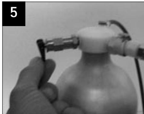
5. Confirm the blue lever on the pressure bleed valve is pointing downward in the closed position.
