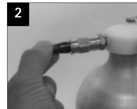
2. Open the pressure bleed valve on the Hi-Float® reserve cylinder to release the pressure from the cylinder. The valve is in the open position when the blue lever is in the horizontal position.
