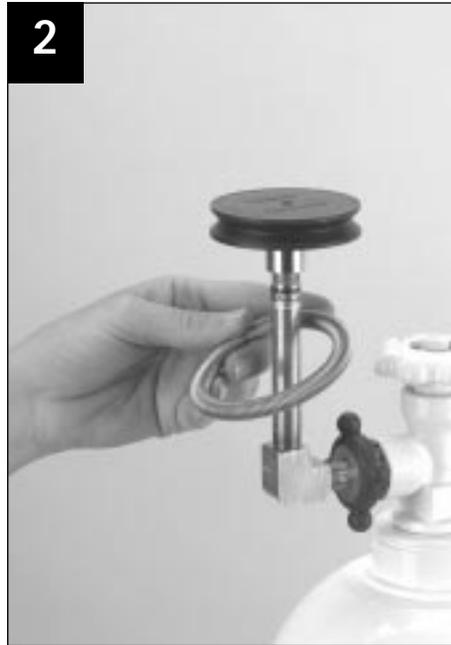
**2.** Remove the holding spring from disc. Leave the spring hanging from the inflator next to the handtight connection.
