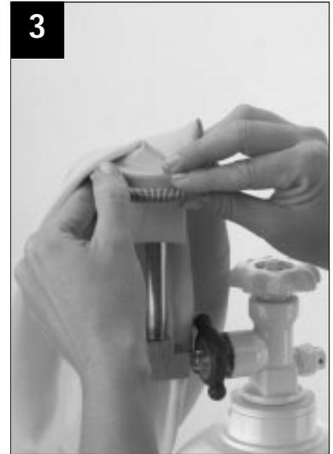
**3.** To secure the balloon to the inflator, stretch the neck of the large balloon over the disc and replace the holding spring in the groove. For best results, place the spring near the end of the neck of the balloon to allow for ease in tying the balloon. (See step 5 below.)
