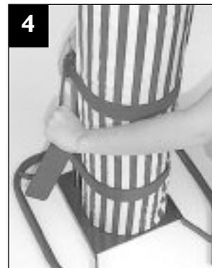
4 Roll the cylinder into the safety stand until it is touching the upright supports. Orient the cylinder valve outlet so it is facing to the left. Place bottom Velcro® safety belt around cylinder and through loop. Tighten belt securely. Repeat with top belt. Cylinder should be very tightly attached to stand.
