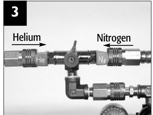
Connect the primary hoses to the Quick Switch by snapping the primary regulator hose from the helium tank into the side marked "He" and the primary regulator hose from the nitrogen tank into the side marked "N2".
