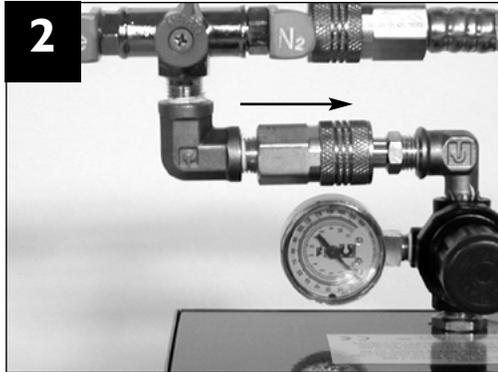
Attach the Quick Switch to either the back of Duplicator 2 or Dual Sizer by snapping on the press fit connection.
