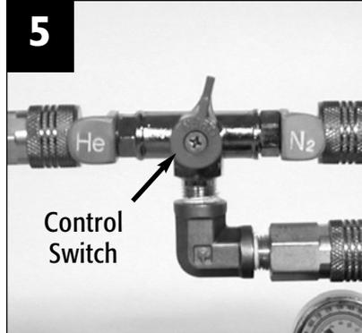
To switch between helium and nitrogen, simply use the control switch to open the flow of gas.
