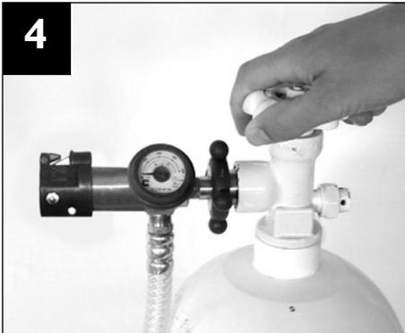
Slowly open the cylinder valve. Make sure the valve is fully opened. The cylinder pressure will read on the gauge located on the primary regulator. The inlet pressure will read on the adjustable regulator gauge located on the back of the unit.
