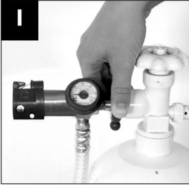
Hand-tighten the helium regulator to the helium tank. Make sure the cylinder is properly secured in a safety stand or wall bracket prior to attaching the regulator.
