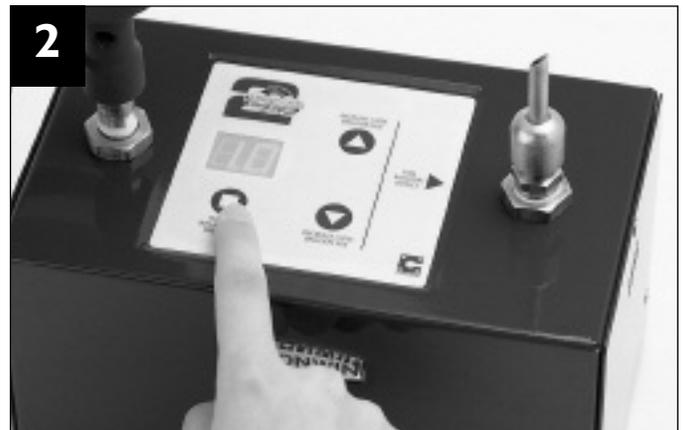
Cycle the system until all the pressure has been released from the unit. Disconnect the supply hose and adjustable regulator from the back of the unit. Remove regulator from the cylinder. Unscrew the latex inflating outlet and pack the Duplicator 2 and all components in the protective carrying case.
