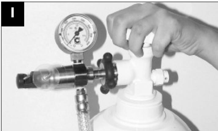
Close the cylinder valve/shut off the air compressor.
