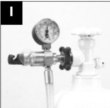
Hand-tighten the regulator to a helium or nitrogen cylinder. Make sure the cylinder is properly secured in a safety stand or wall bracket prior to attaching the regulator.
