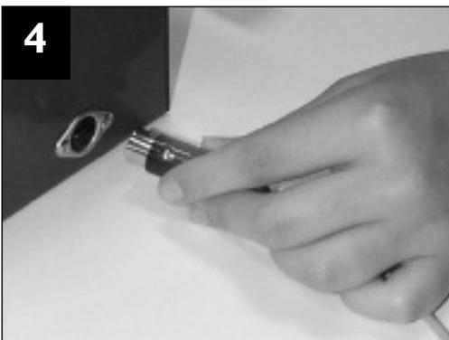
Plug the foot pedal (if included) into the side of the unit.
