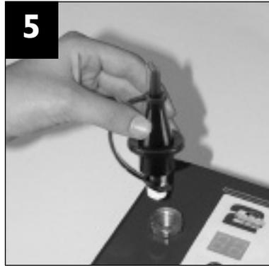
Hand-tighten the latex inflating outlet to the Duplicator 2. Accessory outlets available are featured on the back page.
