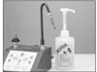
The hand-tight HI-FLOAT® Outlet enables the user to inflate balloons filled with HI-FLOAT® neck up. This prevents any HI-FLOAT® from getting into the Duplicator 2.
