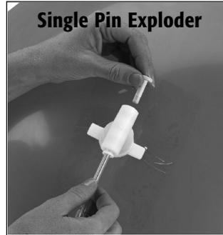
Cut the air line with scissors at each interval where an exploding balloon is required. Press the end of the air line into the Quick-Fit Connector until it reaches the back of the fitting, approximately 1/2 inch. Pull on the air line to insure that the Quick-Fit Connector properly grips the line. Attach the Single-Pin Exploder at the end of the air line. Keep the Plug in place when terminating the line at the exploder or remove the Plug to run a continual line of exploders.
