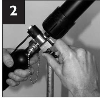
2. The angle of the cannon barrel can be adjusted to achieve different effects. Select the proper angle for the event and tighten the wing nut to hold the barrel in place. Use a heavy weight at the base of the column. Before loading the Confetti Cannon with confetti and covering the conduit with balloons, test fire the cannon prior to the event to insure the column is properly secured. The cannon will kick when fired.
