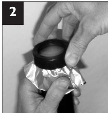
2 Use a foil balloon to seal the barrel. Cut a 6" radius circle out of a foil balloon (Use a popped or scrap balloon). One circle will provide two pieces of foil material. Place one foil circle over the end of the barrel and screw the barrel into the cannon base.
