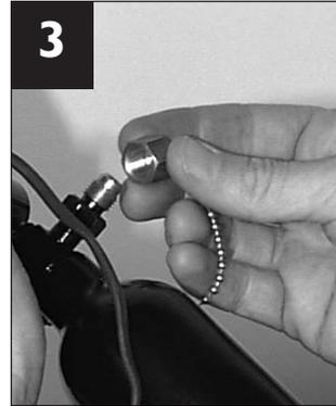
3 Remove the cap from the filling outlet on the cannon. The cap has a bead chain attached to insure that it doesn't get misplaced.
