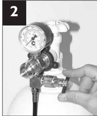
2 Make sure the bleed valve on the regulator is closed before filling the cannon cylinder.
