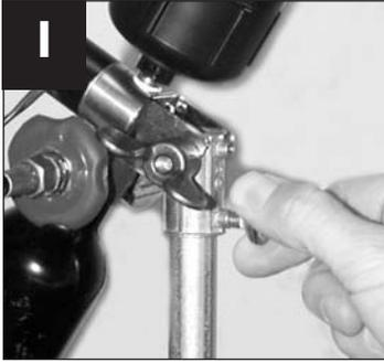
1. The rigging mount, located at the bottom of the barrel fits a 1/2" electrical conduit. Place the conduit into the mount and firmly tighten the thumb screw to secure the cannon in place.
