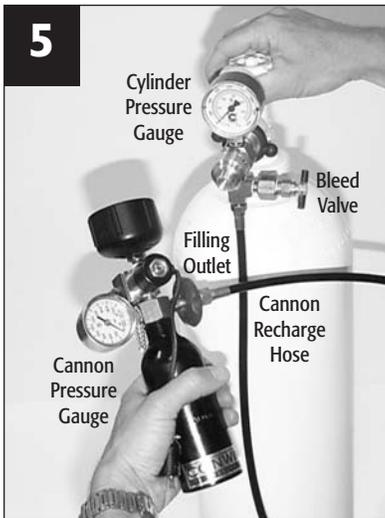
5 Slowly open the cylinder valve. The preset regulator on the filling hose will automatically recharge the cannon with the proper amount of gas. The gauge on the cannon will read approximately 1,000 psi when the cannon is fully charged. Close the cylinder valve. Open the bleed valve to release the pressure from the filling hose. Remove the filling hose from the filling outlet and tighten.
