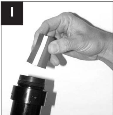
1 Screw the barrel on to the cannon. Remove the cap ring from the barrel and fill the barrel with confetti. If using bundled confetti, be sure to remove the rubber bands before placing them in the barrel. To avoid confetti from clumping, do not tightly pack the confetti in the barrel.
