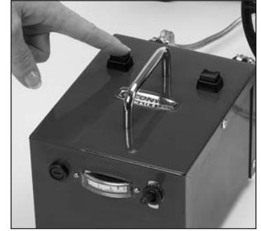
On cue, **push and hold down** the Control Box detonator button until the cannon has completely fired. For best results, wait for approximately 2 seconds between pressing the first and second button. This will prolong the air time of the confetti.
