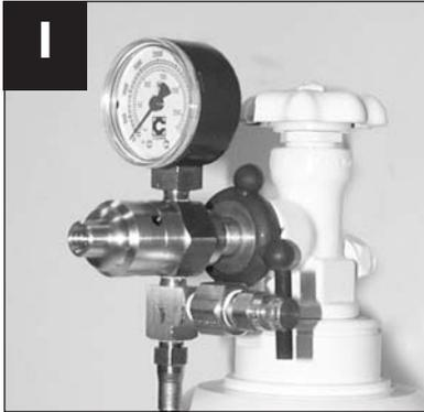
1 Hand-tight connect the regulator to a helium or nitrogen cylinder. The cylinder must have a minimum of 1,000 psi gas pressure to properly charge the cannon.
