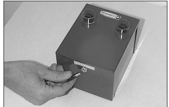
Plug the Control Box Battery Charger into a 110-volt electrical outlet. Plug the other end into the back of the Control Box to charge it. **Important!** Recharge the battery with the Battery Charger for at least 8 hours prior to use. The battery can be recharged at any level.
